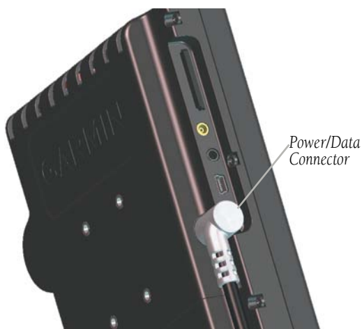
GPSMAP 695/696 and Power/Data Connector
